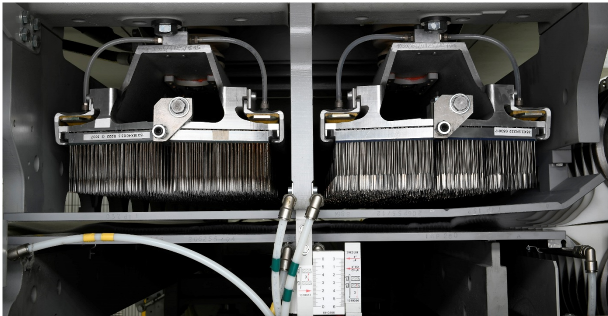
SFD (self-feeding device) system on a pre-needleloom to feed a wide range of fiber batts
